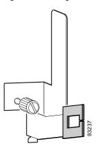
Figure 31 Multiport Line Card Cable-Management Bracket
